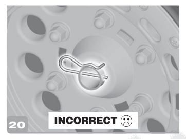
• If the clip is upside down or not through both holes in the axle, you have not assembled it properly. Please remove the clip and go back to step 18.
